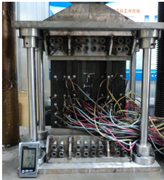
Figure 3. Gripped stiffened composite panels for compressive load experiment.
