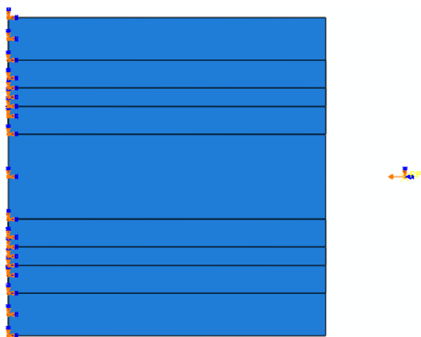
Figure 4. Boundary conditions of stiffened composite panels in the finite element model under compressive load.
