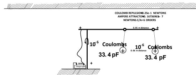
**Figure 4.** Two non-oscillating spheres, on an orientable Greek capital letter  $\Gamma$  shaped support, holding similar or opposite and equal magnitude charges, affected by their orientation, time and date on the Earth, due to that instant's all known velocities of Earth: rotation and orbital velocity of the Earth and also Galaxian velocity of 215 km/s of the Sun around the Galactic center.
