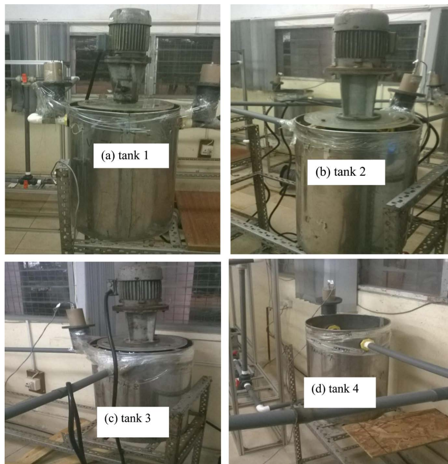
Figure 1. Tanks with different impeller configurations. (a) 1 axial impeller; (b) 2 axial impellers; (c) 2 radial impellers; (d) no impeller no baffle.
