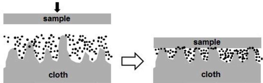
**Figure 1.** Effective abrasive particles in the polishing interface.
