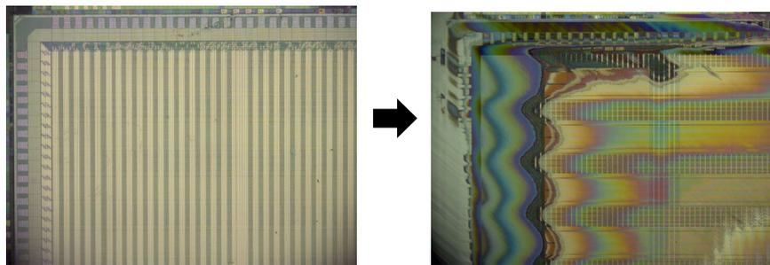
**Figure 5.** Surface pattern evolution during polishing process.
