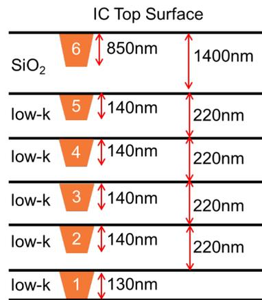
**Figure 3.** Film stacking structure of a typical 40 nm IC chip.
