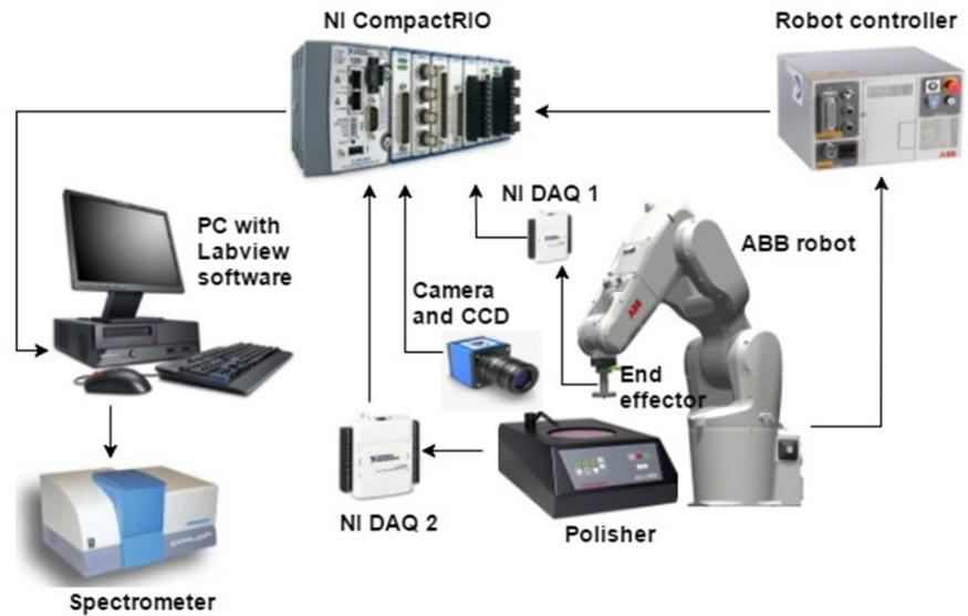
**Figure 4.** Smart polishing system configuration.
