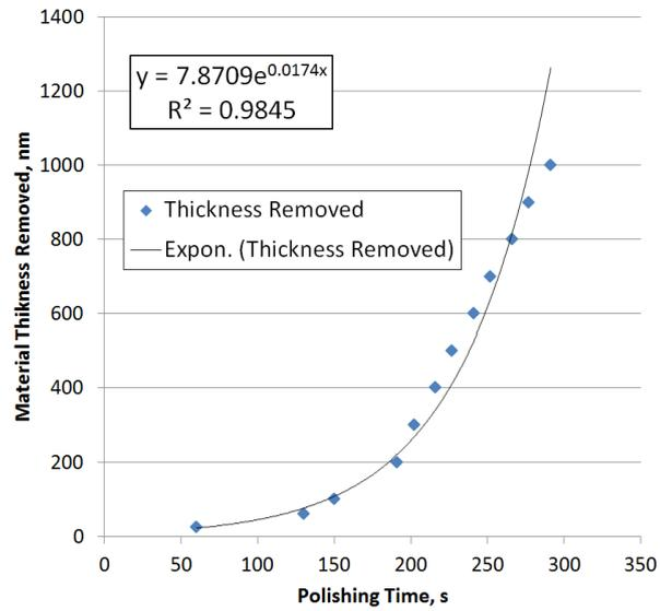
**Figure 2.** Predicted polishing time for removing a certain amount of material.
