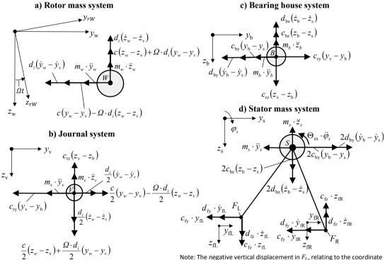
Note: The negative vertical displacement in  $F_L$ , relating to the coordinate  $z_{fL}$ , is considered by the direction of the vertical forces in  $F_L$ , so  $z_{fL}$  has to be described in the differential equation by:  $z_{fL} = -z_s + \varphi_s \cdot b$
