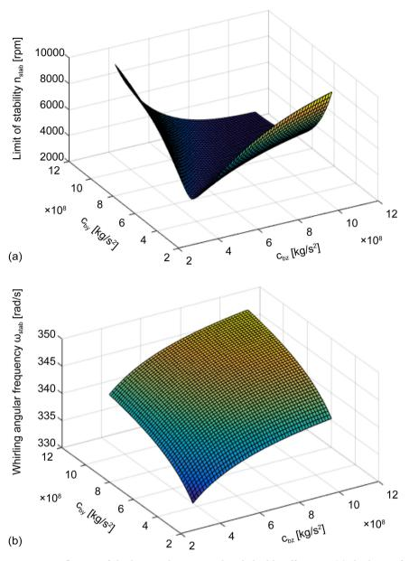
**Figure 11.** Influence of the bearing housing and end-shield stiffness on (a) the limit of stability  $n_{stab}$  and on (b) the whirling angular frequency  $\omega_{stab}$  for a rigid foundation.
