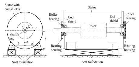
**Figure 1.** Special kind of rotating machine with rotor, roller bearings, bearing housings, end-shields and stator, mounted on a soft foundation.
