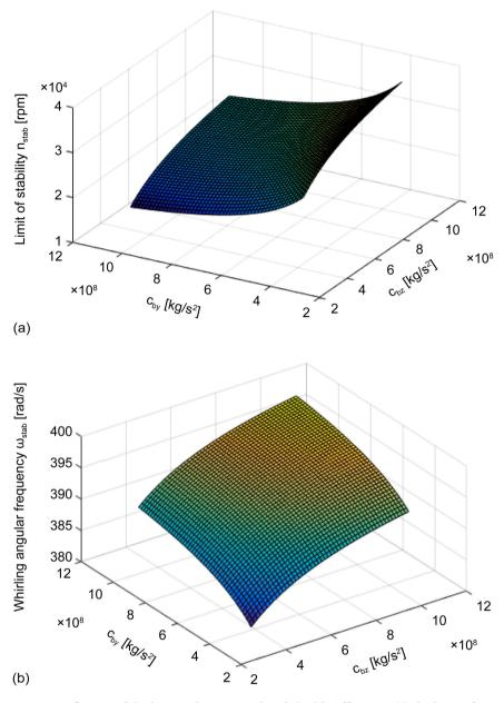
Figure 9. Influence of the bearing housing and end-shield stiffness on (a) the limit of stability  $n_{stab}$  and on (b) the whirling angular frequency  $\omega_{stab}$ , for the rated soft foundation (Table 1).
