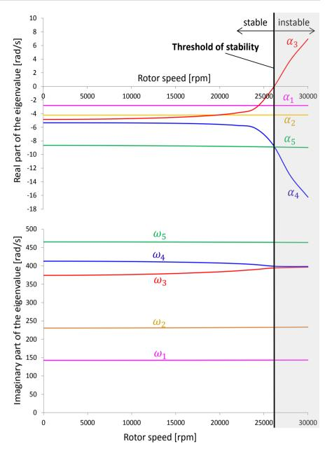
Figure 5. Eigenvalues, depending on the rotor speed and threshold of stability.
