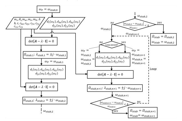
Figure 4. Flow diagram to derive the threshold of stability.
