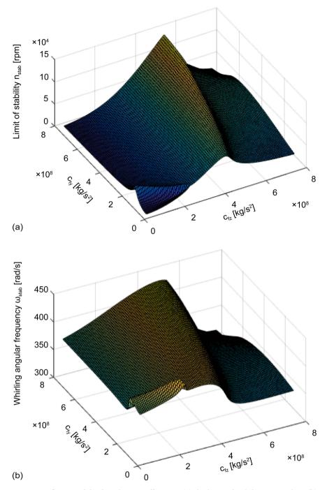
**Figure 7.** Influence of the foundation stiffness on (a) the limit of stability  $n_{stab}$  and on (b) the whirling angular frequency  $\omega_{stab}$ .
