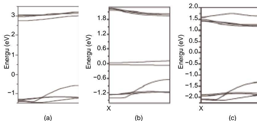
**Figure 4.** Diagram for electronic band structure (a) SiNW, (b) SiNW with N doped, (c) SiNW with -OH group.
