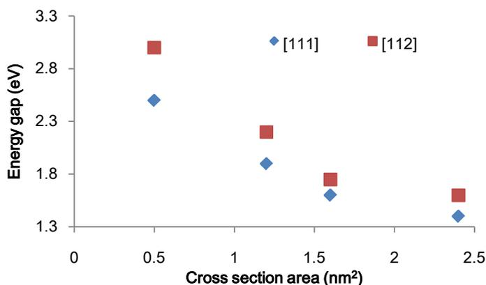
**Figure 3.** Band gap of the SiNWs versus the cross-sectional area, blue dots is for [111], brown for [112].
