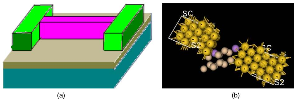
**Figure 1.** (a) Schematic of SiNW model, (b) view of SiNW with dopant in virtual NanoLab.
