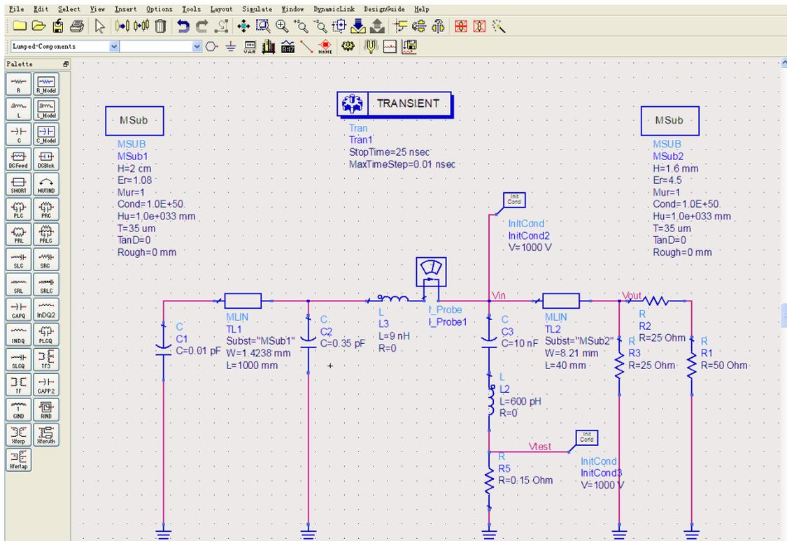
Figure 3. Equivalent circuit of cable discharge.
