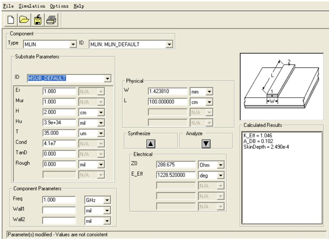
Figure 2. Simulation parameters of microstrip line.
