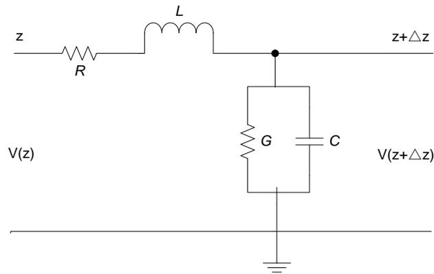
Figure 1. Element analysis of a cable.
