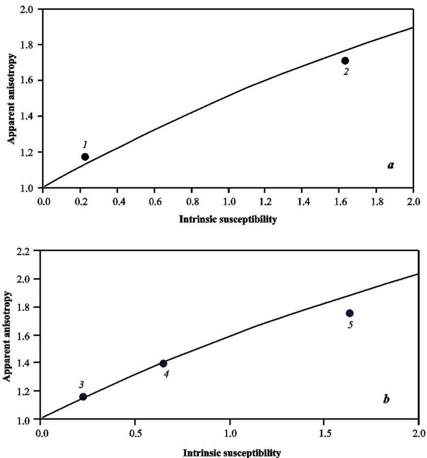
**Figure 5.** Theoretical curves of apparent anisotropy ( $A_a$ ) versus intrinsic susceptibility ( $\kappa$ ) with length-to-diameter ratio of the magnetic layer ( $p$ ) of 0.1250 (a) and 0.0625 (b). Black dots are corresponding experimental results of measured anisotropy using artificial samples in [5]. The volume fraction of magnetic layer material ( $v_m$ ) is  $1/2$ .
