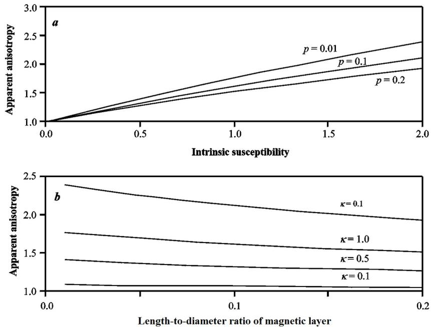
**Figure 4.** Theoretical curves of apparent anisotropy ( $A_a$ ) versus: (a) intrinsic susceptibility ( $\kappa$ ), and (b) length-to-diameter ratio of the magnetic layer ( $p$ ). The volume fraction of magnetic layer material ( $v_m$ ) is  $1/3$ .
