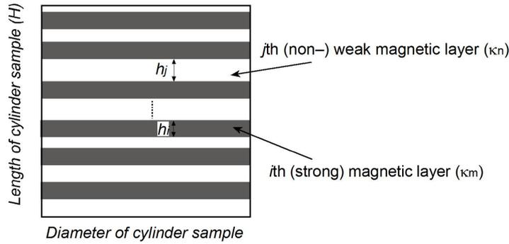
Figure 3. Schematic section of a cylindrical BIF sample.
