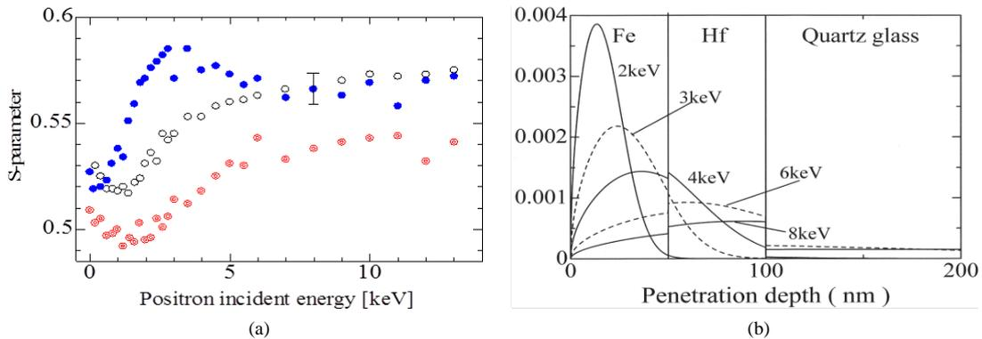
**Figure 1.** (a)  $S$ -parameter vs. incident positron energy for the bilayer Fe (50 nm)/Hf (50 nm); (b) The positron implantation profiles in the bilayer Fe (50 nm)/Hf (50 nm) at some incident energies.
