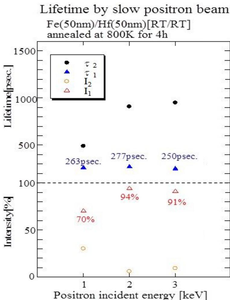
**Figure 3.** The positron annihilation lifetimes and those intensities vs. the incident positron energy for the bilayer Fe (50 nm)/Hf (50 nm) after annealing for 4 hours at 800 K.
