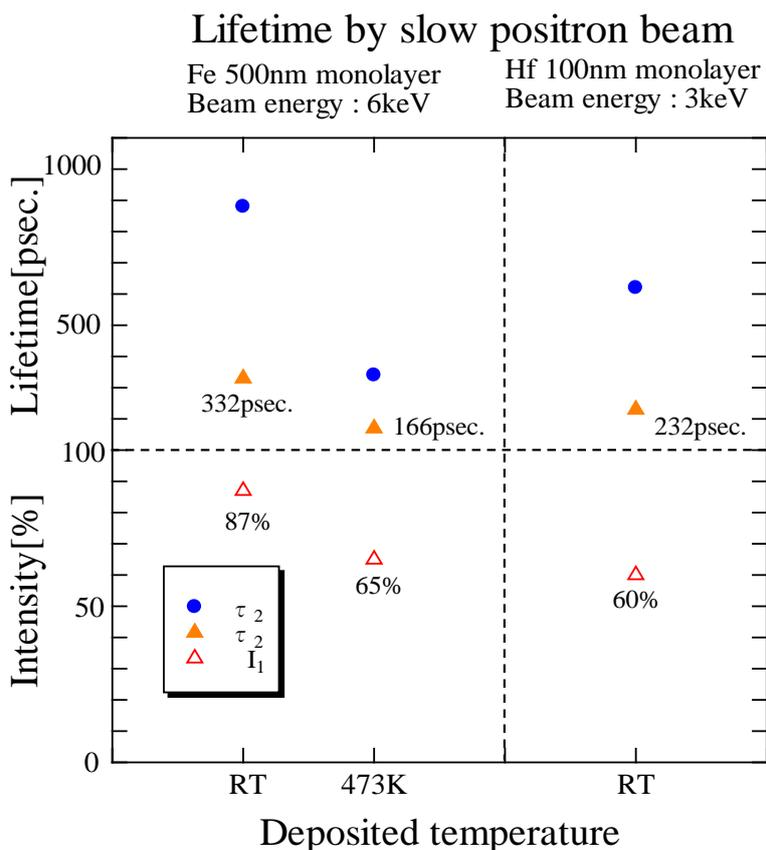
**Figure 2.** The positron annihilation lifetimes and those intensities in the thin Fe film of the thickness 500 nm at room temperature and 473 K, and the lifetimes and intensities in the thin Hf film of the thickness 100 nm at room temperature.
