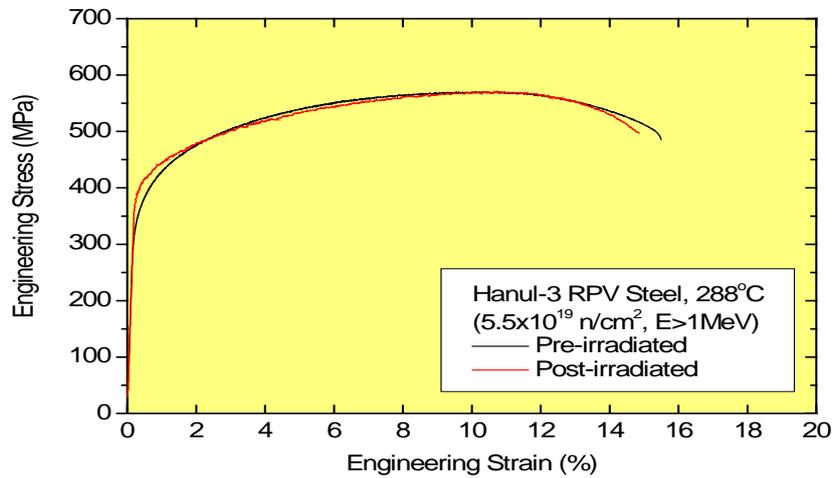
Figure 5. Tensile strength of RPV steel [2].
