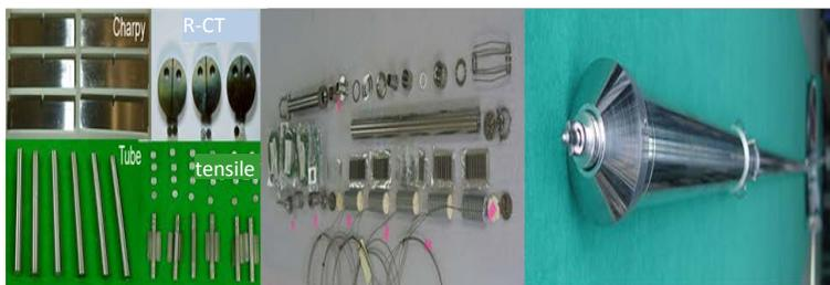
**Figure 2.** Standard capsule, parts and specimens.
