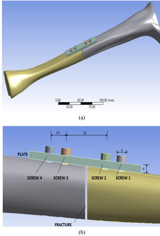
**Figure 2.** (a) Numerical model (b) Dimensions of the plate and screws.
