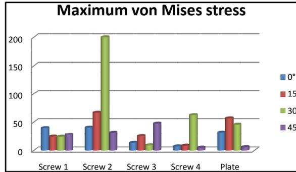
**Figure 5.** Maximal von Mises stress on the plate and the screws (×10<sup>7</sup> GPa).
