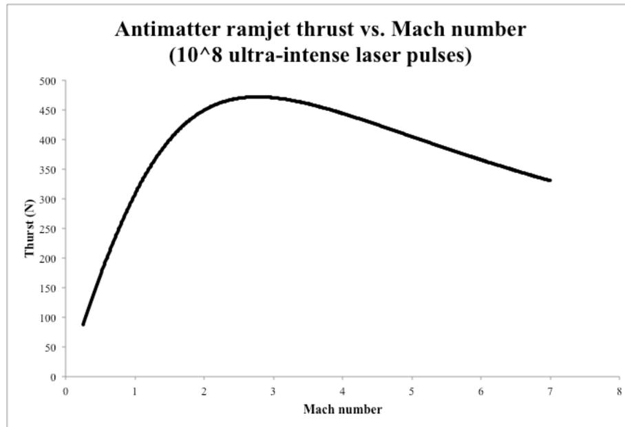
**Figure 1.** Antimatter ramjet thrust as a function of flight Mach number.
