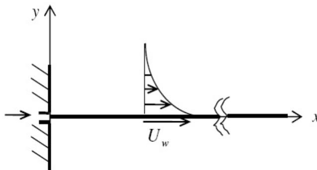
**Figure 1.** The physical model of the boundary layer on a continuously moving surface.
