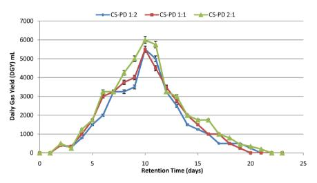
**Figure 3.** Progress curve showing the Daily Gas Yield (DGY) for the co-digestion of Corn Stalk (CS) with Poultry Droppings (PD) at different mixing ratios with a retention time of 24 days.
