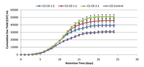
**Figure 4.** Progress curve showing the Cumulative Gas Yield (CGY) for the co-digestion of Corn Stalk (CS) and Cow Dung (CD) at different mixing ratios with a retention time of 24 days.
