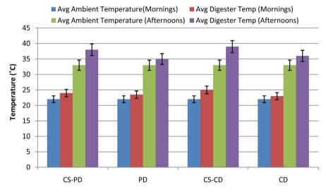
**Figure 7.** Measurement of Temperature from the co-digestion of Corn Stalk (CS) with Poultry Droppings (PD), Cow Dung (CD) at different mixing ratios. Note: \*Initial ambient temperature in the mornings and average ambient temperature between 11 am and 5 pm is  $35^{\circ}C \pm 2^{\circ}C$ . Initial average digester temperature was ambient temperature.
