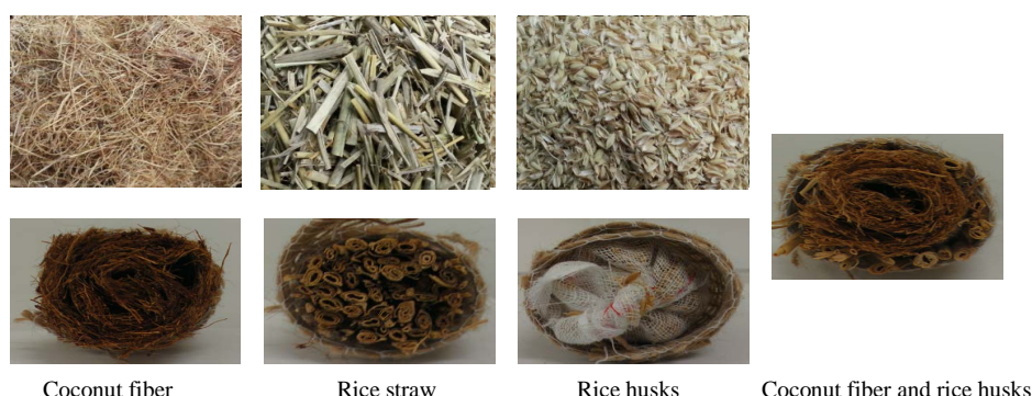
Figure 1. Four types of BCD materials derived from various agricultural byproducts.
