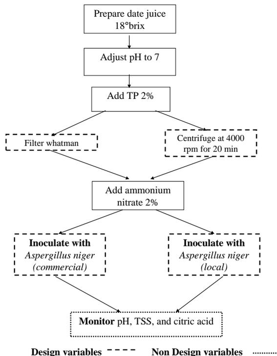
**Figure 2.** A process flow diagram showing design variables and non design variables.
