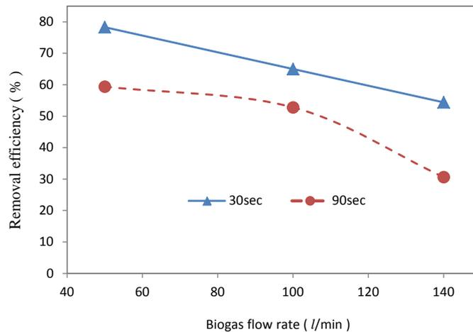
**Figure 4.** The removal efficiency of H<sub>2</sub>S content for biogas in different biogas flow rate without circulating water system.
