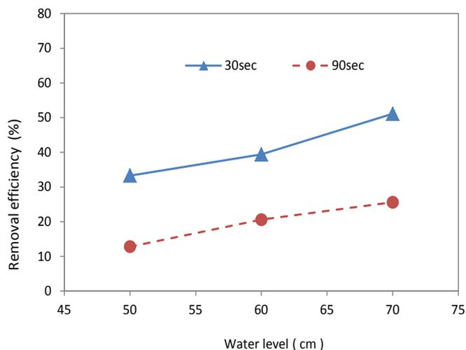
**Figure 3.** The removal efficiency of H<sub>2</sub>S content for biogas in different water level without circulating water system.
