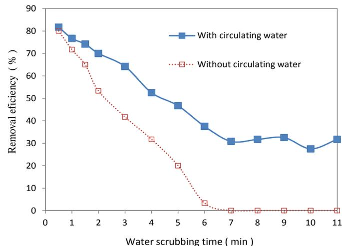
**Figure 5.** The relationship of removal efficiency of H<sub>2</sub>S content for biogas and water scrubbing time.
