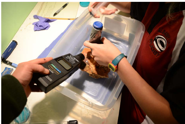
Figure 2. Utilizing the Cen-Tech digital photo tachometer DT-838 to measure the revolutions per minute during drilling of the temporal bone utilizing the guide drill bit and countersink drill bit.
