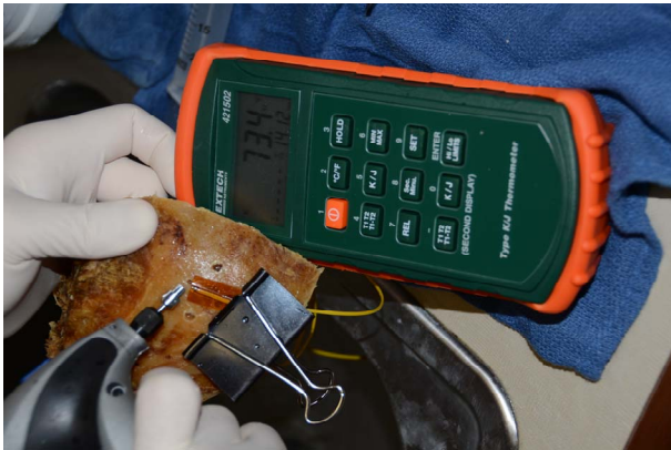
Figure 3. Utilizing the Extech dual input digital thermometer model 421502 to measure the temperature of the temporal bone adjacent to the drill hole while drilling with the guide drill and countersink drill.
