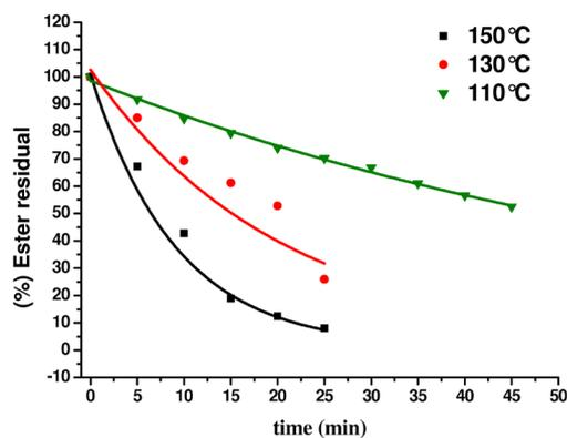
**Figure 1.** Effect of temperature on the hydrolysis of sunflower oil.
