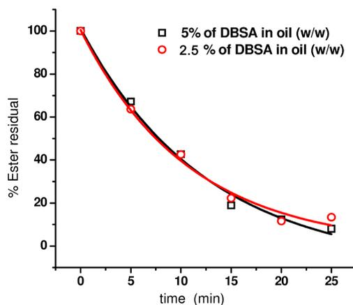
**Figure 2.** Effect of catalyst level on the hydrolysis of sunflower oil using 40/60 (w/w) water-to-oil ratio at 150°C.
