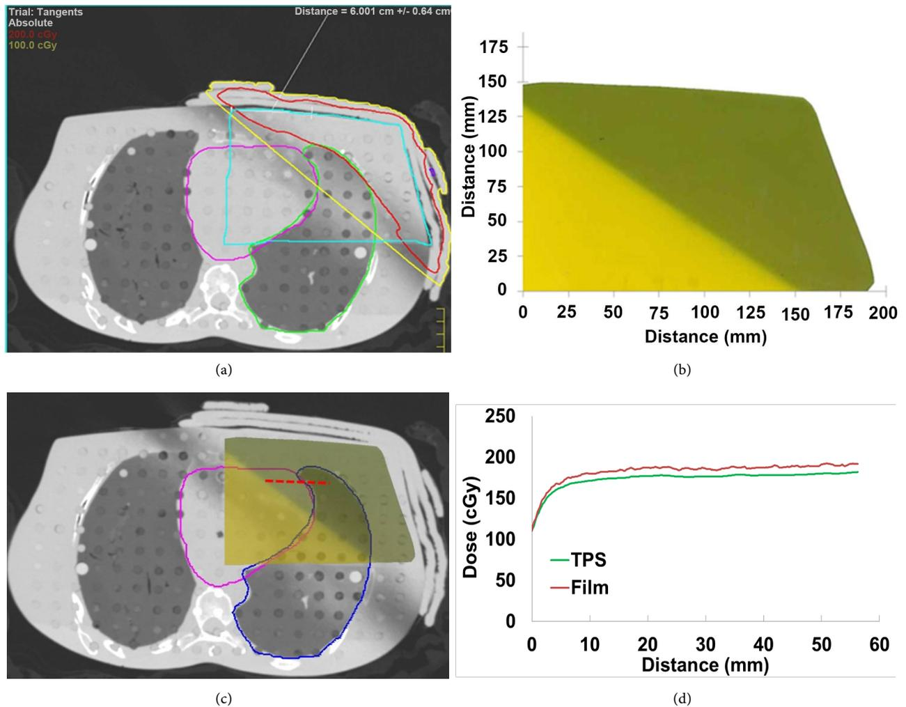
**Figure 8.** (a) Plane from planning CT, structure highlighted in blue is the embedded film; (b) Irradiated film was scanned; (c) Registration between **Figure 8(a)** and **Figure 8(b)**. The RED dashed line shows the position where dose in left lung and heart was extracted; (d) Dose profile in heart and left lung along the RED dashed line drawn in **Figure 8(c)**.
