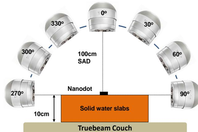
**Figure 2.** Schematic diagram of angular dependence on nanoDots. The gantry angles were at 30°, 60°, 90°, 330°, 300° and 370°.
