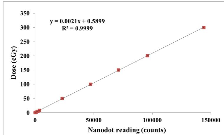
**Figure 4.** NanoDot calibration curve for 6 MV photon beam.
