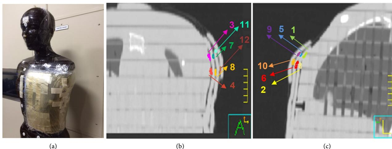
**Figure 3.** (a) Femal ART phantom; (b) Axial view of the scanned ART phantom; (c) Sagittal view. Positions of 12 nanoDots are labeled.
