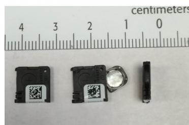
**Figure 1.** AnanoDot, material used is Aluminum oxide doped with Carbon ( $\text{Al}_2\text{O}_3;\text{C}$ ) with  $1.2 \text{ mm}$  thickness and  $5 \text{ mm}$  diameter encased in  $10 \text{ mm} \times 10 \text{ mm} \times 1.8 \text{ mm}$  light tight plastic holder.
