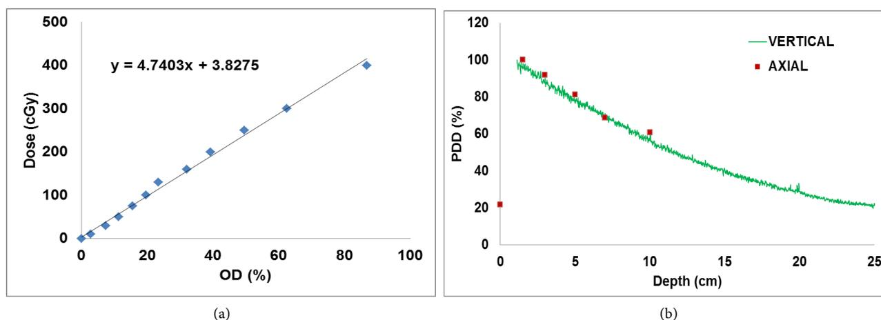
**Figure 6.** (a) Film calibration curve; (b) PDD comparison with film is vertical and axial to photon beam.
