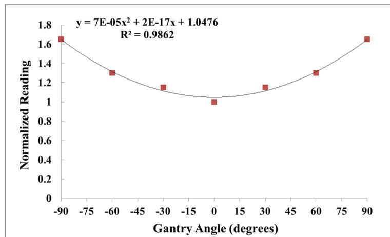
**Figure 5.** Response of nanoDot with the variation of beam direction.
