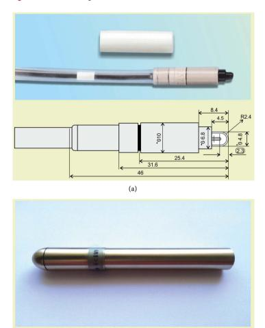
**Figure 2.** (a) Scanditronix-Wellhöfer CC04 compact ion chamber and its diagram; (b) Brass-alloy "build-up" cap [19].
