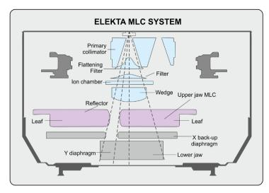
Figure 1. The head diagram of Elekta (TM) Linear accelerator head [18].
