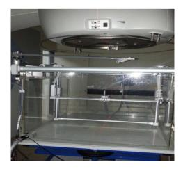
Figure 3. The in-air output measurement set-up.
