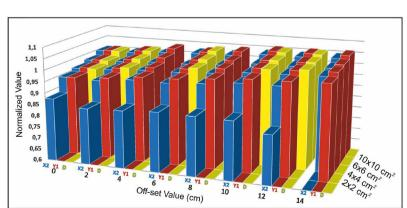
The in-air output measurement values for different off-set distances and indicated fields were obtained (Table 1). For calculating  $S_c$  factor for them, the in-air
