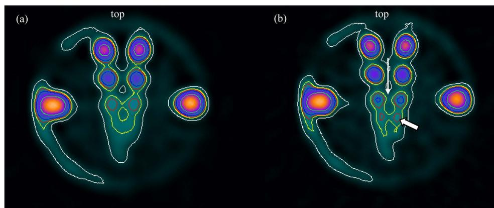
**Figure 3.** Transverse images of hot regions insert with (a)  $0.35 \text{ cycles}\cdot\text{cm}^{-1}$  and (b)  $0.45 \text{ cycles}\cdot\text{cm}^{-1}$  cut-off frequencies and an order 5 of filter.
