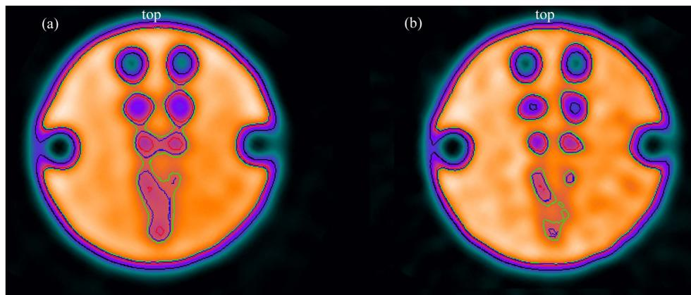
**Figure 5.** Transverse images of cold regions insert with (a)  $0.35 \text{ cycles}\cdot\text{cm}^{-1}$  and (b)  $0.45 \text{ cycles}\cdot\text{cm}^{-1}$  filter cut-off frequencies and an order 5.
