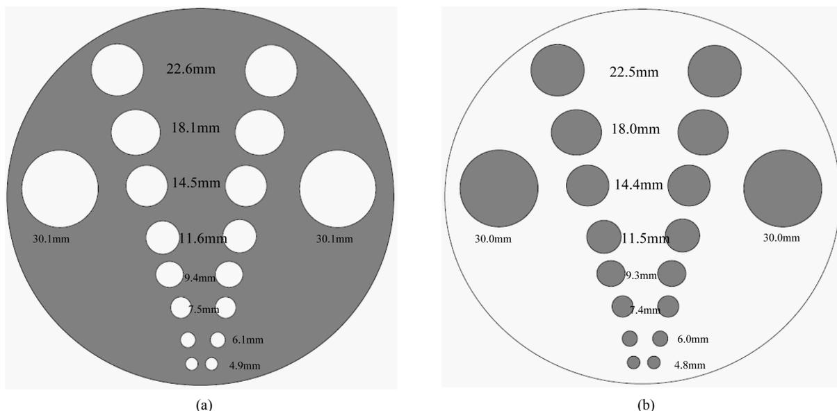
**Figure 1.** Schematic cross-sectional views of (a) hot regions insert, and (b) cold regions insert.
