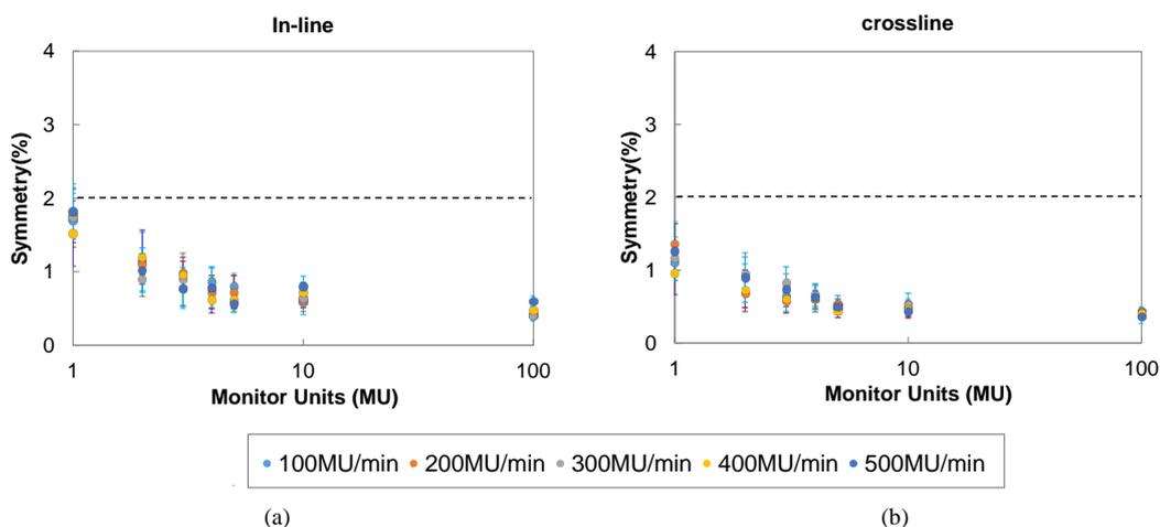
**Figure 4.** Calculated symmetries of the (a) in-line and (b) crossline profiles in a  $(10 \times 10)$  cm<sup>2</sup> field versus the MU setting. Results are plotted for several dose rates. The error bars represent 1 standard deviation based on five measurements. Dashed lines represent the 2% symmetry variation.
