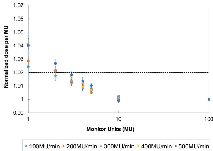
**Figure 2.** Relative delivered dose per MU in a (10 × 10) cm<sup>2</sup> field versus the MU setting. Results are plotted for several dose rates. The error bars represent 1 standard deviation based on five measurements. Dashed lines represent the 2% dose variation.
