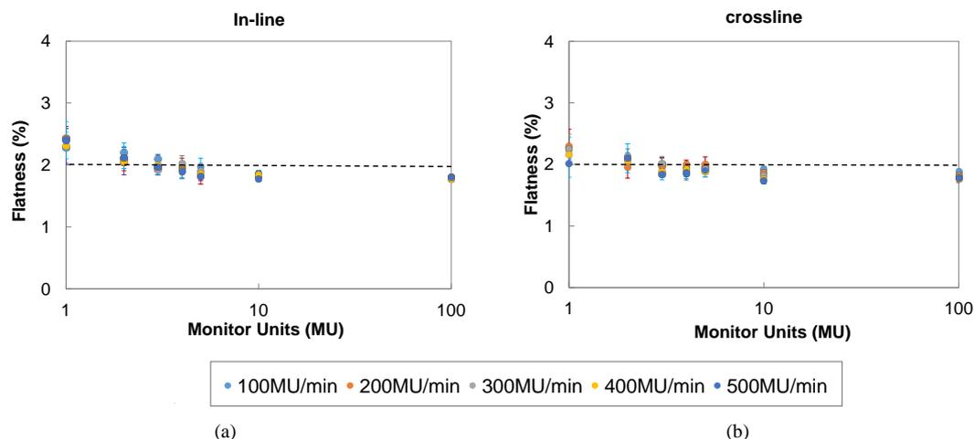
**Figure 5.** Flatness of the symmetry, calculated for (a) in-line and (b) crossline profiles in a  $(10 \times 10)$  cm<sup>2</sup> field versus the MU setting. Results are plotted for several dose rates. The error bars represent 1 standard deviation based on five measurements. Dashed lines represent the 2% flatness variation.
