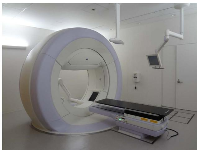
**Figure 1.** Photograph of the Vero4DRT system. The basic structure is the O-ring with diameter of about 350 cm. The gantry which is located inside of the O-ring can be rotated  $\pm 180^\circ$  around the isocenter, and the O-ring itself can be rotated  $\pm 60^\circ$  around its vertical axis through the isocenter.
