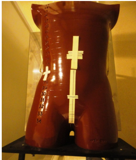
Figure 4. Alderson Rando phantom.
