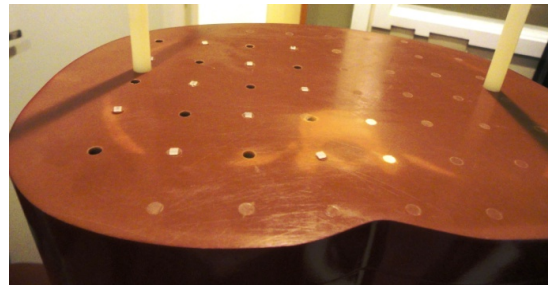
Figure 5. Slice with TLDs and holes [9].
