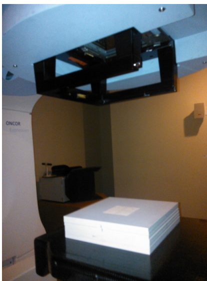
Figure 3. Experimental arrangement for the characterization of TLDs using a solid plate.
