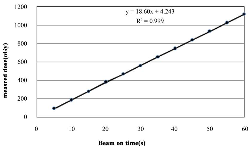
**Figure 2.** The response of linearity of dose and beam on time.
