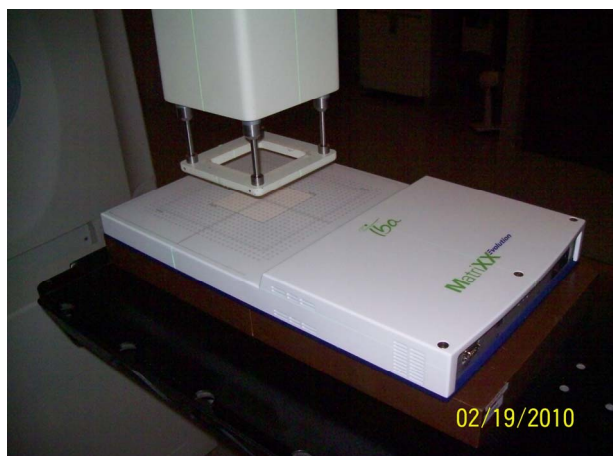
Figure 1. MatriXX setup on a linac treatment tabletop. A proper thickness of Solid Water would be placed on the surface during measurement.
