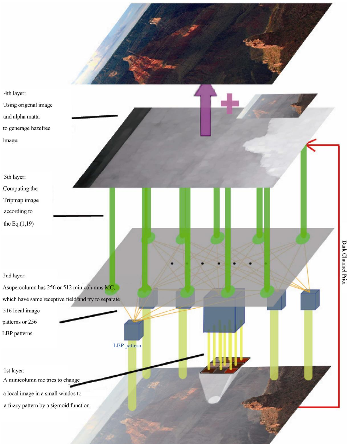
**Figure 2. A 4 layers' structure of a columnar organization of V1 for haze-background separation.**
