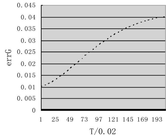
Figure 10. Simulating fuzzy logical and-or by changing thresholds of neural cells. The X-axis is the threshold value divided by 0.02, the Y-axis is errG. The real line is perrAndq between  $I_1 \oplus_f I_2$  and  $\bar{V}_i$ , and the dot line is the perrorq between  $I_1 \oplus_f I_2$  and  $\bar{V}_i$ .
