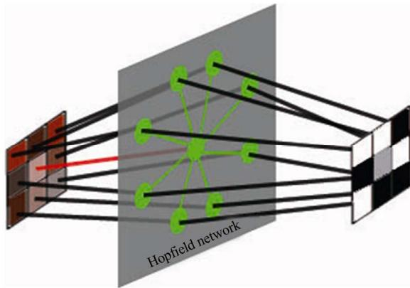
**Figure 3.** Every 1<sup>st</sup> layer minicolumn tries to change local images into binary texture patterns, for a 3×3 small window, a minicolumn in the 1<sup>st</sup> layer contains 9 Hopfield neurons, and every neuron focuses only one pixel.
