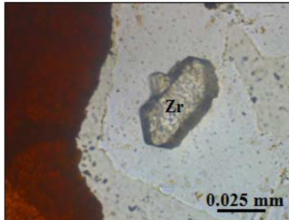
**Figure 10.** Photo micrograph showing detrital zircon under the polarizing microscope (Zr: zircon).
