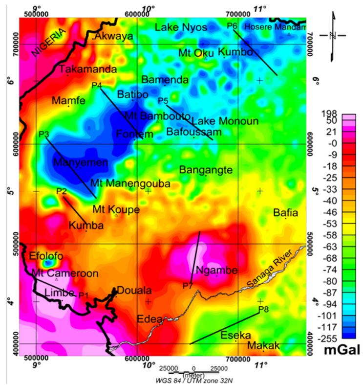
Figure 6. Bouguer anomaly map of the study area derived from EGM2008, dashed lines are profiles.
