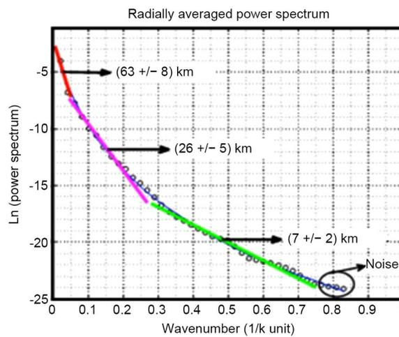
**Figure 16.** Power spectrum versus frequency for profile P<sub>5</sub> (Bafoussam region).
