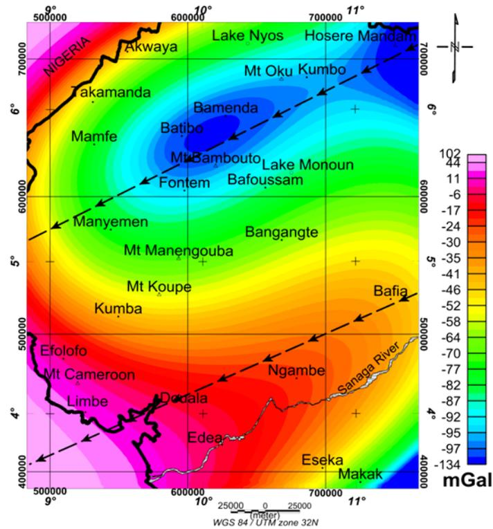
Figure 9. Third-order regional anomaly map from EGM2008, arrows representing the orientation of gradient.
