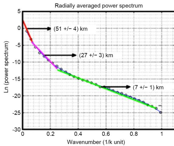
**Figure 15.** Power spectrum versus frequency for profile P<sub>4</sub> (Fontem, Mamfe region).
