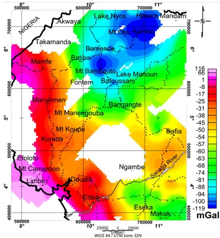
Figure 3. Bouguer anomaly map from existing land gravity data.
