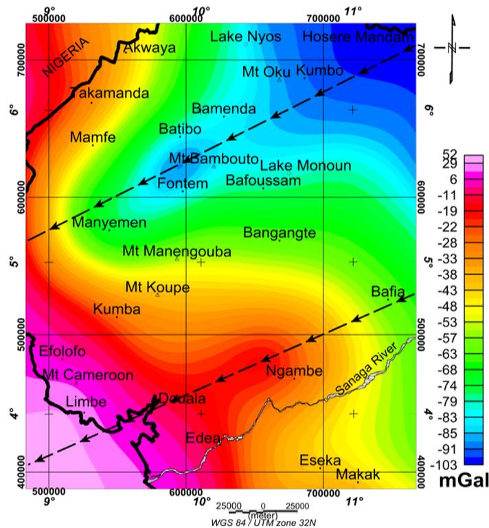
Figure 10. 30 km upward continued regional anomaly map from EGM2008, arrows representing the orientation of gradient.
