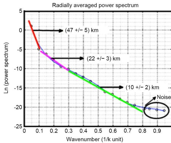
Figure 12. Power spectrum versus frequency for profile P<sub>1</sub> (Mount Cameroon).
