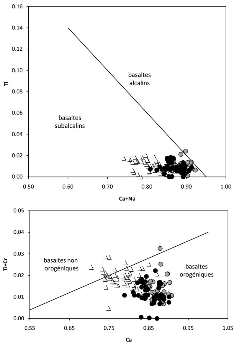
**Figure 4.** CPX (clinopyroxene) location in the Ca + Na-Ti diagram of Letterier *et al.* [33].
