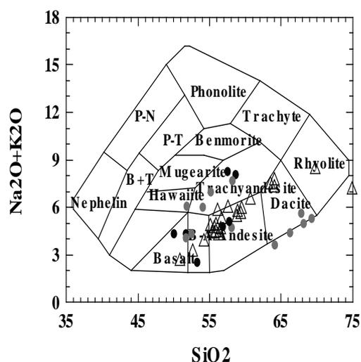
Figure 5. Calc-alkaline volcanic rocks in the  $\text{Na}_2\text{O} + \text{K}_2\text{O} - \text{SiO}_2$  diagram.
