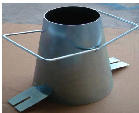
Photo 3. Slump cone mold.
