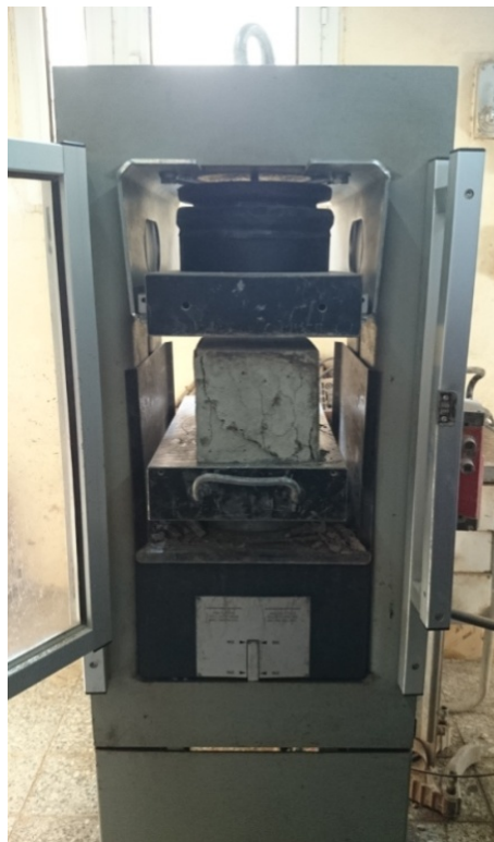
Photo 2. Compressive strength machine.
