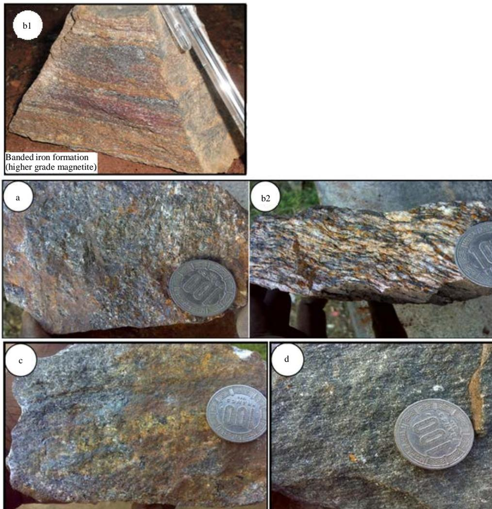
**Figure 2.** (a) Sample of itabirite; (b1, b2) Banded Iron Formation (BIF); (c) Sample of iron-bearing gneiss; (d) Sample of amphibolites.
