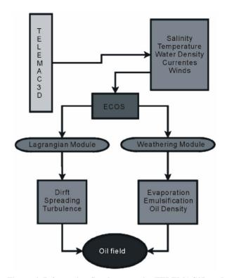
Figure 4. Information flux between the TELEMAC3D and the ECOS model.
