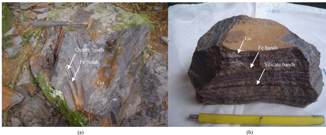
Figure 4. (a) Intensely folded oxide facies BIF with alternative silica and iron banding, stained by goethite (Go). (b) Banded silicate facies BIF sample with some goethite coating.
