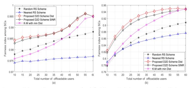
**Figure 5.** Load balancing index among SCs versus number of offloadable users. (a) The first scenario: semi-balanced load among the SCs. (b) The second scenario: significant imbalanced existing load among SCs.
