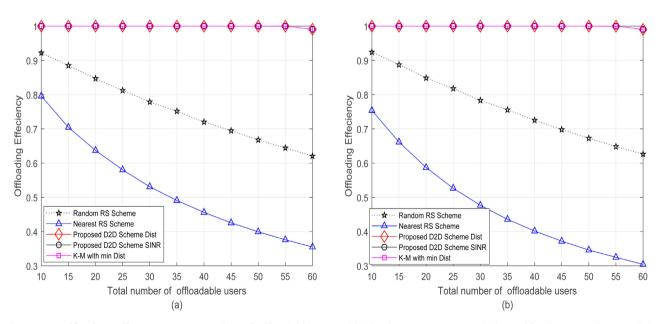
**Figure 6.** Offloading efficiency versus number of offloadable users. (a) The first scenario: semi-balanced load among the SCs. (b) The second scenario: significant imbalanced existing load among SCs.
