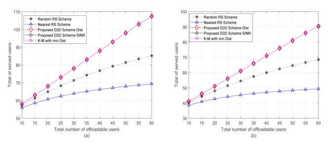
**Figure 4.** Total number of admitted users versus number of offloadable users. (a) The first scenario: semi-balanced load among the SCs. (b) The second scenario: significant imbalanced existing load among SCs.
