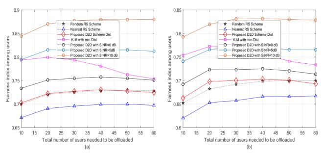
**Figure 7.** Load balancing index among users versus the number of offloadable users. (a) The first scenario: semi-balanced load among the SCs. (b) The second scenario: significant imbalanced existing load among SCs.
