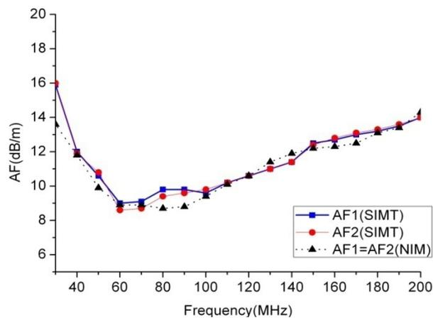
**Figure 3.** AF of biconical antennas calibrated.
