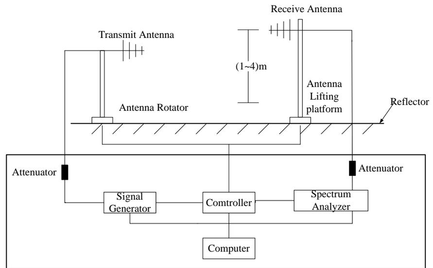
**Figure 1.** AF measurement system.
