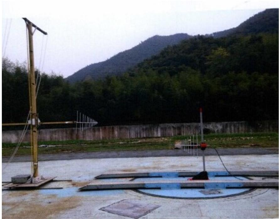
**Figure 2.** AF measurement system on OATS.
