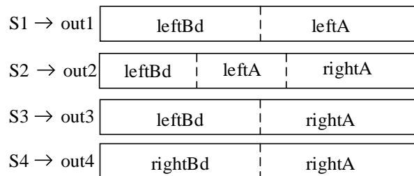
Figure 5. The combination output of left and right shifter. The FSM is set as (1) S1: Dout is the combination of leftA and leftBd which from the left shifter. (2) S2: Dout is the combination of leftBd and leftA from the left shifter, and rightA from right shifter. (3) S3: combination of leftBd and rightA. (4) S4: combination of rightBd and rightA. (5) Idle: no operation.
