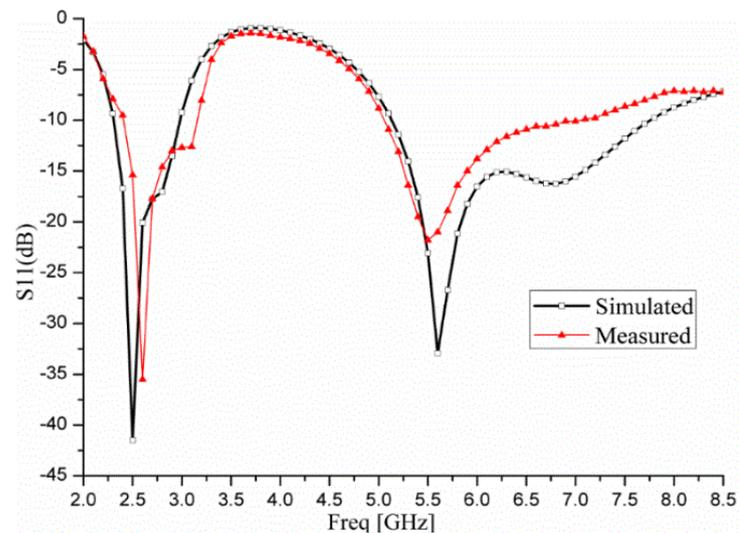
**Figure 10.** Simulated versus measured RL.
