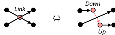
Figure 2. Planarization of a spatial structure, i.e. the removal of a crossing, is achieved by cutting the rear connection and inserting a pair of Aktons instead called Down and Up.
