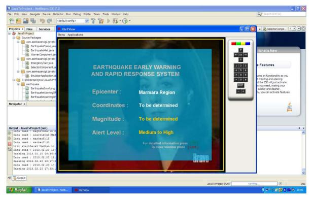
Figure 6. "Medium to High risk" (possibly 3.5 or more on the Richter Scale) *P-wave* based live earthquake early warning information, which appears as a pop-up window on the TV screen. At this point, the exact magnitude and epicenter of the earthquake are not known.
