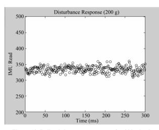
Figure 12. Roll axis hover test response for 200 g load.
