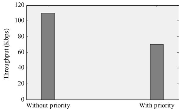
**Figure 5. Throughput of flows 2-4, with flow 1 as high priority and without priority.**
