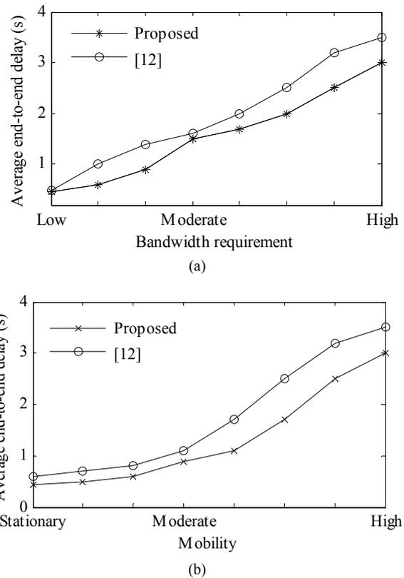
**Figure 7. Average end-to-end delay vs. bandwidth requirement (a), and average end-to-end delay vs. mobility (b).**
