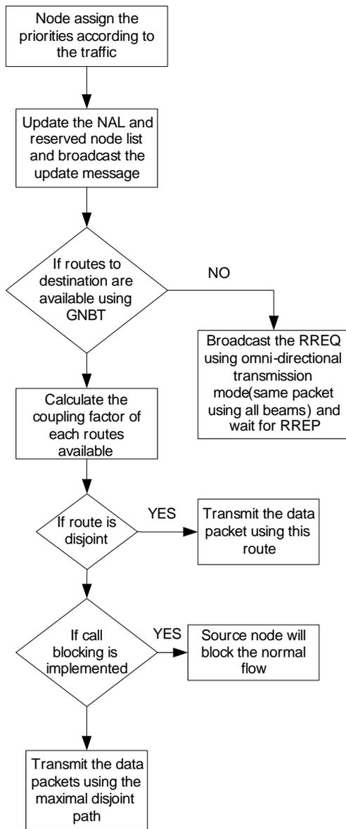
**Figure 3. Flow chart of QoS routing protocol for without and with call blocking.**
