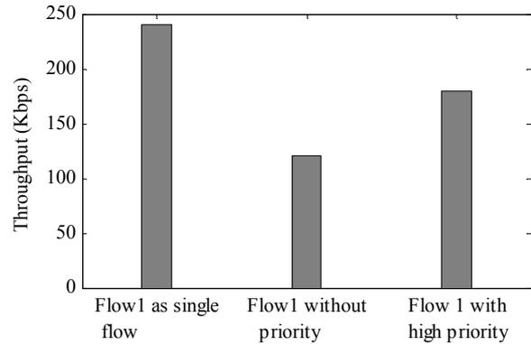
**Figure 4. Performance of throughput of flow 1 when only single flow 1 and four flows (1-4) are present in the network with and without priority.**
