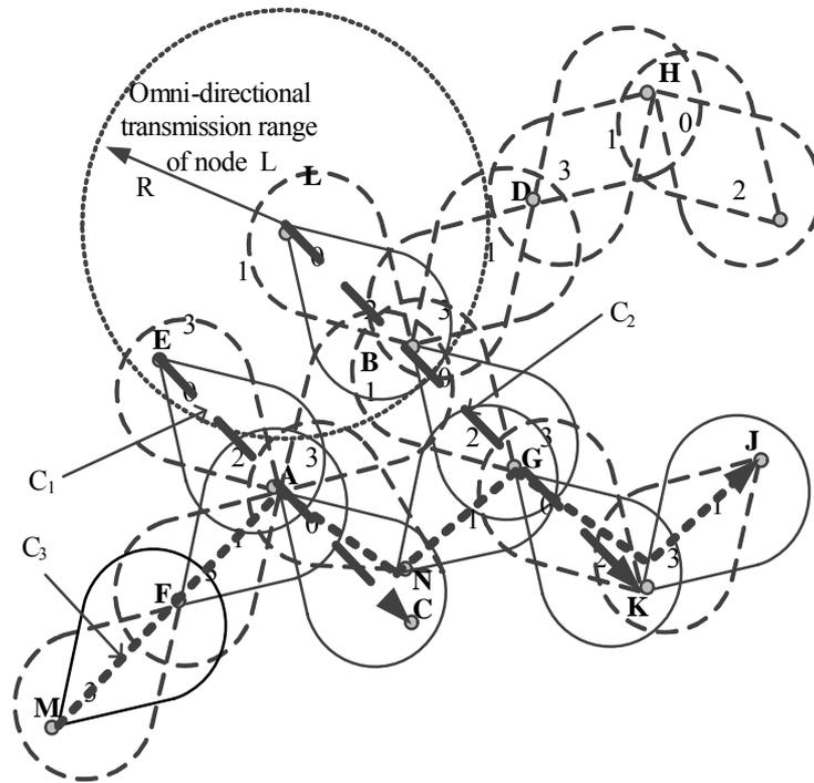
Figure 1. Simultaneous transmission through coupled routes using directional antenna.
