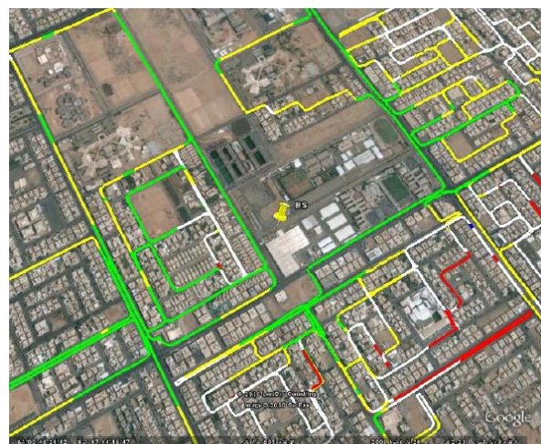
Figure 2. A sample signal map for the collected data for one site. The color legend are Green: RSSI > -70 dBm, Yellow: -80 \leq RSSI < -70 dBm, White: -89 \leq RSSI < -80 dBm, Red: RSSI < -90 dBm.
