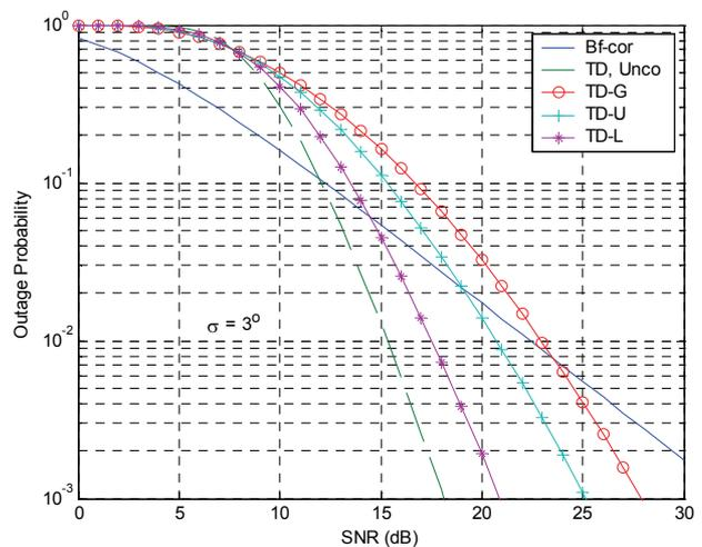
**Figure 3.** Outage probability for Transmit diversity and beamforming systems for UCA; mean AOA  $\theta = 0^\circ$ ,  $\sigma = 3^\circ$ ,  $C_{out}(p) = 3$ ,  $M = 4$ .
