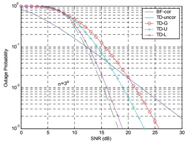
**Figure 2.** Outage probability for Transmit diversity and beamforming systems for ULA; mean AOA  $\theta = 0^\circ$ ,  $\sigma = 3^\circ$ ,  $C_{out}(p) = 3$ ,  $M = 4$ .
