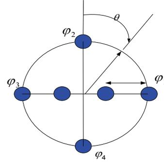
**Figure 1. Four element ULA and UCA antenna array configuration at the base station.  $R$  is radius of circular array and  $d$  is the spacing between array elements,  $d = 2R/3$ .**
