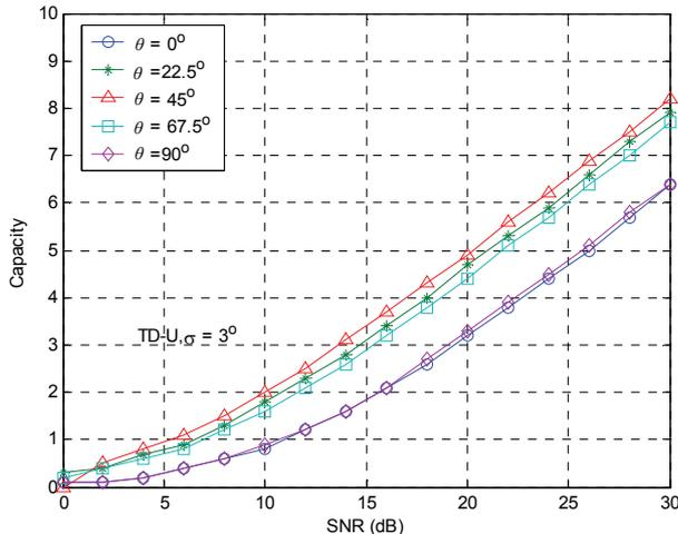
**Figure 7. Outage capacity for Transmit diversity for UCA with uniform AOA;  $\sigma = 3^\circ$ ,  $M = 4$ ,  $p = 2\%$ .**
