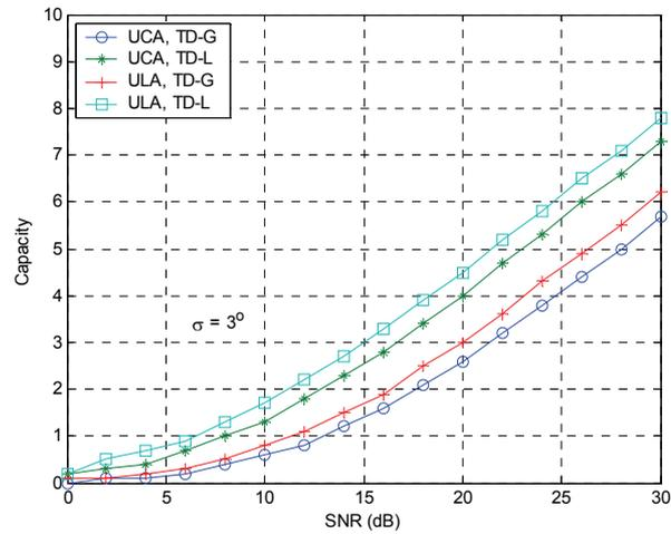
**Figure 5. Outage capacity for Transmit diversity for ULA/UCA; mean AOA  $\theta = 0^\circ$ ,  $\sigma = 3^\circ$ ,  $M = 4$ ,  $p = 2\%$ .**
