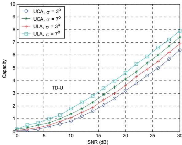
**Figure 4. Outage capacity for Transmit diversity for ULA/UCA with uniform AOA;  $\theta = 0^\circ$ ,  $M = 4$ ,  $p = 2\%$ .**
