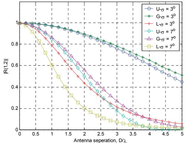
**Figure 6. Spatial envelop correlation between antenna 1 and 2 for ULA; mean AOA  $\theta = 0^\circ$ ,  $M = 4$ .**
