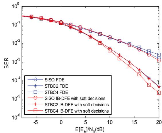
Figure 1. Uncoded BER results for the SC-FDE.
