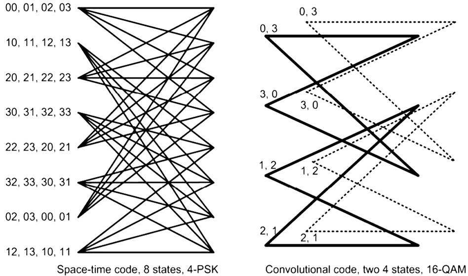
Figure 1. Trellis diagram of block space-time code and convolutional code.
