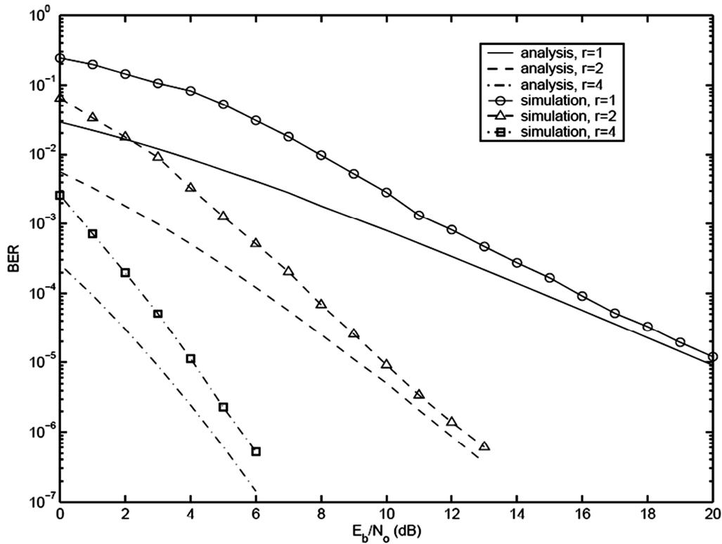
Figure 3. Block space-time code, two transmit antennas, 8 states, 4-PSK, 1, 2 and 4 receive antennas, Rayleigh.
