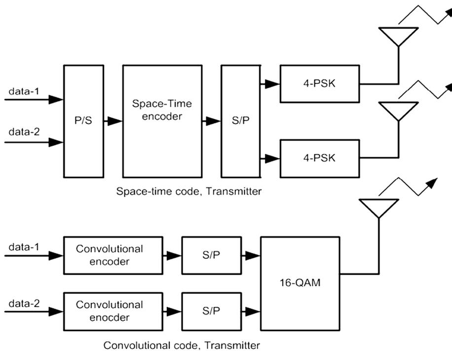
Figure 2. Transmitter structures.
