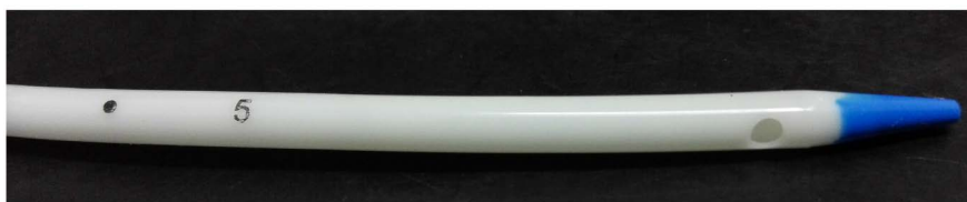
Photo 1. The object of distance from the inner venous port to the inner arterial port.
