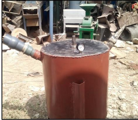
**Plate 1.** Biogas digester.
