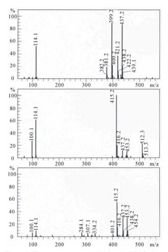
Figure 4. The mass spectra recorded for the HPLC chromatogram of Tuxidrin. The upper figure shows the massspectrum of pholcodine, the middle figure shows the mass spectrum of pholcodine-N-oxide, and the bottom figure shows the mass spectrum of a substance tentatively identified as 10-hydroxy-pholcodine. Conditions used for MS are described in the Materials and Methods section.
