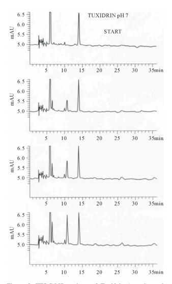
Figure 3. HPLC-MS analyses of Tuxidrin (experimental conditions described in the text). The upper chromatogram shows the Tuxidrin just off the production line, beneath is the same sample analyzed after 9, 27 and 62 days. The peaks with their retention times are as follows: pholcodine at 6 min, pholcodine-N-oxide at 6.5 min, 10-hydroxy-pholcodine at 11 min, and ephedrine at 14 min.
