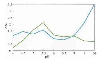
Figure 2. The percentage of oxidation products present in, calculated as a percentage of the total amount of pholcodine. The blue line is the concentration of pholcodine-N-oxide and the green line is the concentration of 10-hydroxy- pholcodine. Temperature: 60°C. Duration of accelerated degradation: 62 days.
