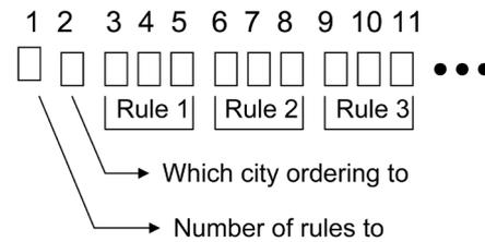
**Figure 1.** A rule based encoding for the traveling salesman problem.
